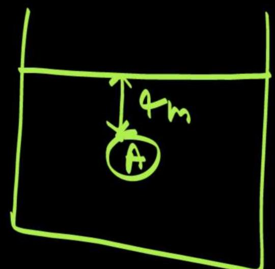
PA = 9 9 1 X 4 = 39.24 KP9 Q: ) In the stability of floating bodies, the stable equilibrium is attained if the meta centre (M) point the centre of gravity (G) (DFCCIL Civil JE 10-11-2018)
